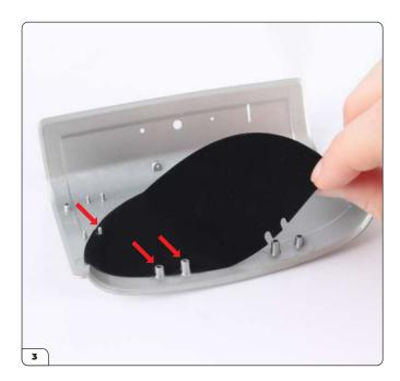
Start to press the carpet onto the boot lid, making sure to fit the holes in the carpet around the pins and screw posts (arrows).
