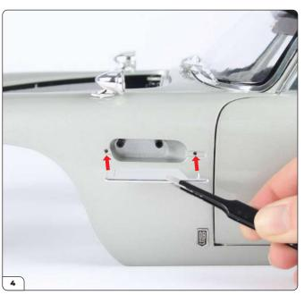
Align the side strake (85-A) with the main body as shown.
