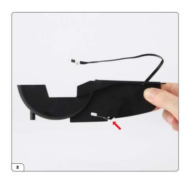
Bend the plug end of the cable so that it comes through the gap as highlighted by the arrow.
