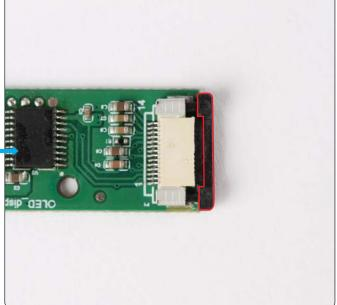
Take the circuit board (92-C) and unlock the socket by sliding the black section out as shown.
