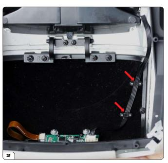
Secure the wire to the boot lid carpet using the two wire brackets (92-F) as shown.
