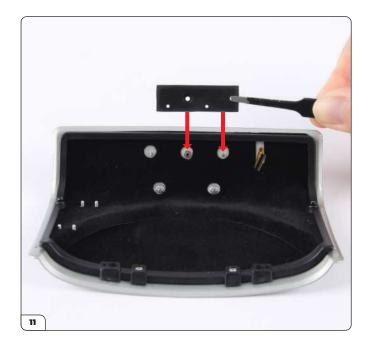
Align the circuit board mount (92-D) with the inside of the boot lid. Press it onto the screw post and pin as shown by the arrows.
