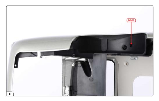
Secure the rear wheel arch with a DS02 screw.
