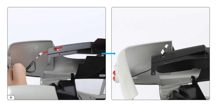
Place the main body upside down on your work surface. Take the rear right wheel arch (87-A) and fit the wire plug (No. 14) through the rectangular hole in the wheel arch.
