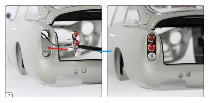
Push the rear light trim into the recess, orienting it with the orange indicator on top. If the wire pushes the brake light out when fitting try using transparent glue to hold the brake light in place.
