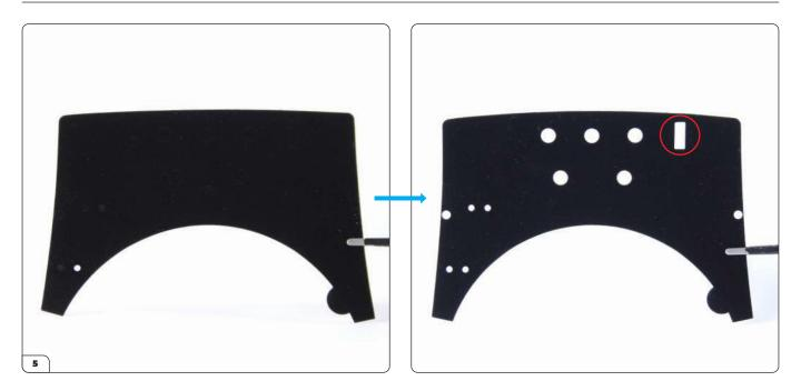
Take boot lid carpet 1 (90-B) and remove the cut out sections from it as shown. If you are using the non-LED number plates, you do not need to remove the rectangular section (circled).
