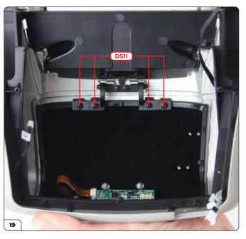
Position the boot lid against the body and secure the boot lid to the hinges using 4x DS11 screws.
