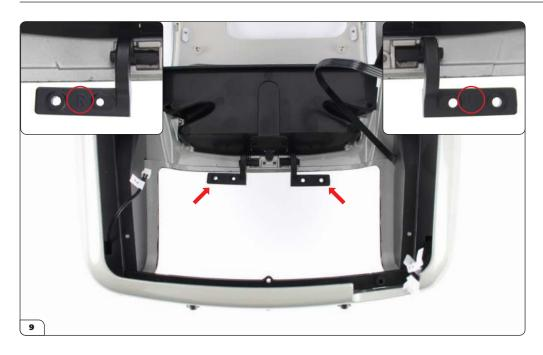
Take the right (89-F) and left (89-E) boot hinges. Position them on the main body as shown. The parts are marked with "R" and "L" (inset images).
