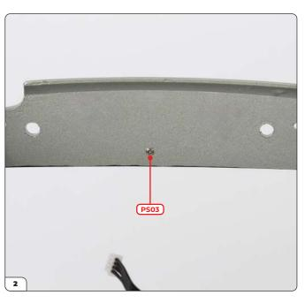
Secure the latch with a PS03 screw.
