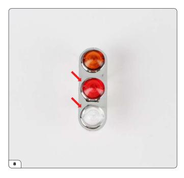
Press the red brake light (85-E) into the middle hole and the transparent reverse light (85-D) into the bottom hole.
