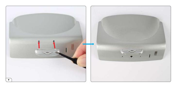
Take the rear number plate light assembly (stage 089) and press it into the two upper holes in the boot lid (stage 091).
