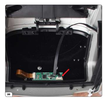
Plug the rear number plate wire (No. 09) into the circuit board.
