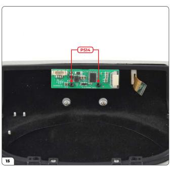
Position the circuit board over the two screw holes then secure it in place with 2x PS14 screws.
